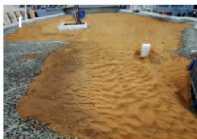
Figure 2 - Comprehensive mobile-bed model using low density model sediments
