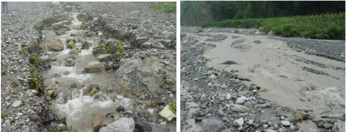
Figure 4 Comparison of Shengou Creek (left) and Hunshui Gully (right) (Shengou: p = 10.34 kg/ms, S_p = 0.285 , g_b = 0.002 kg/ms; Hunshui: p = 10.16 kg/ms, S_p = 0.04 , g_b = 18.9 kg/ms)
