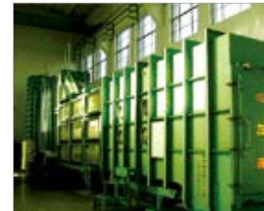
Vacuum tank (vacuum percentage 98.7%; flow discharge 1.0 m³/s)
