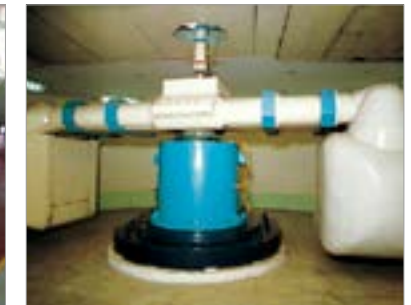
LXJ-4-450g-t geotechnical centrifuge
