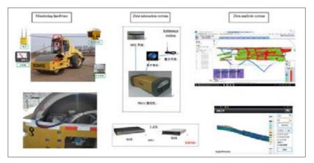
Real-time and intelligent monitoring system for dam filling construction process
