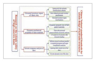
Framework of the research results on seismic safety of high concrete dam
