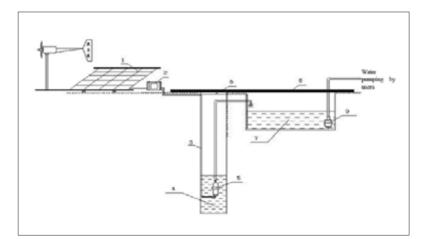
Water supply mode for pastures with wind-solar hybrid power system
