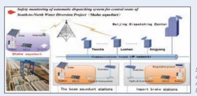
Safety monitoring of automatic dispatching system for central route of South-to-North Water Diversion Project
