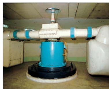
LXJ-4-450g-t geotechnical centrifuge
