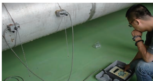
Calibration of clamp-on (externally mounted) ultrasonic flowmeter by using the water flow standard facilities (DN500mm)
