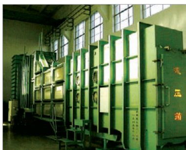
Vacuum tank (vacuum percentage 98.7%; flow discharge 1.0 m)
